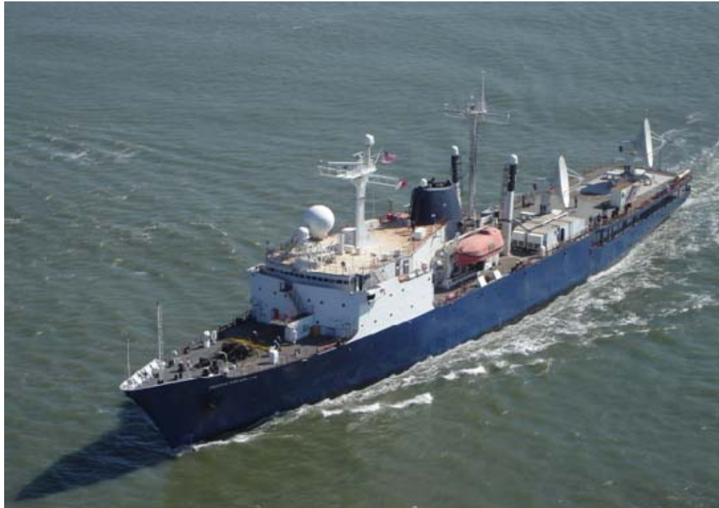
Figure 2. The MV Pacific Collector . The twin 7m dishes of the Transportable Telemetry System are seen in the aft section of the ship (T-AGS-29, n.d.).
