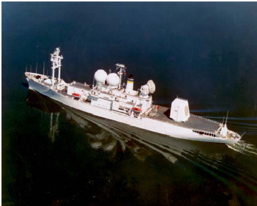
Figure 4. Observation Island : The S-Band phased array is seen on the aft deck, and the X-Band radar is seen atop the house, aft of the smokestack (USNS Observation Island, 2001).
