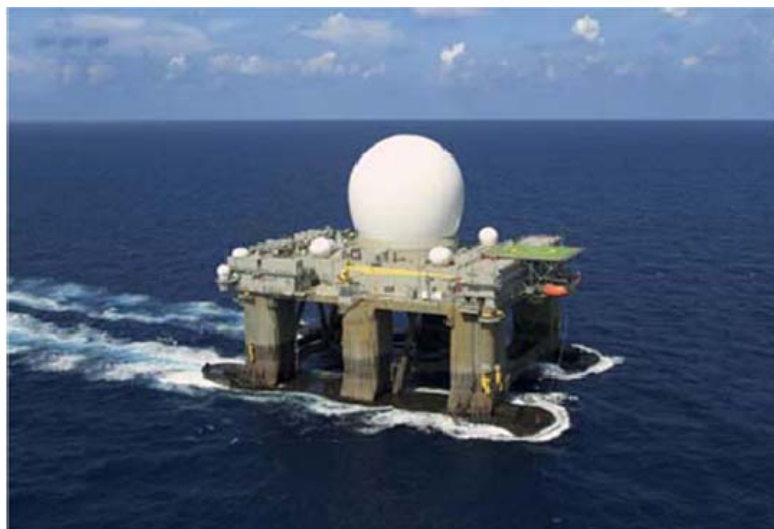
Figure 5. Sea-Based X-Band Radar: The X-Band radar is under the large center dome (SBX, 2007).
