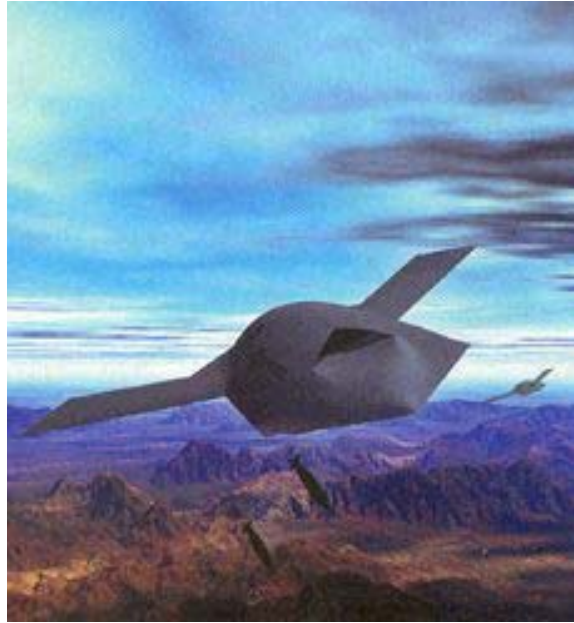
Figure 2. An artist's rendition of the Boeing Unmanned Combat Air Vehicle (UCAV). The UCAV is the next step toward minimizing combat fatalities while supporting two major combat roles: Suppression of Enemy Air Defenses and precision strike. Figure from - [Boeing.com, 2001].
