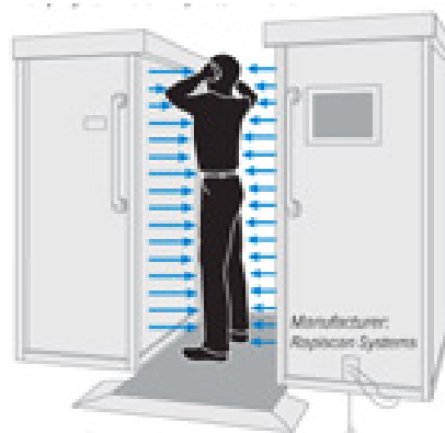
Figure 3. Backscatter scanner (From InterVISTAS, 2007)
