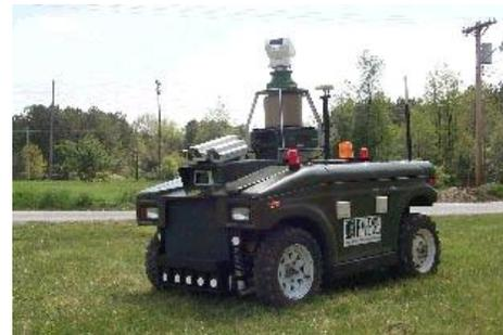
*Mobile Detection Assessment Response System - Exterior (MDARS-E) Autonomously conducts surveillance activities checking for intruders, conducts lock interrogations, and assesses the status of facility barriers, such as the doors of storage bunkers.*
