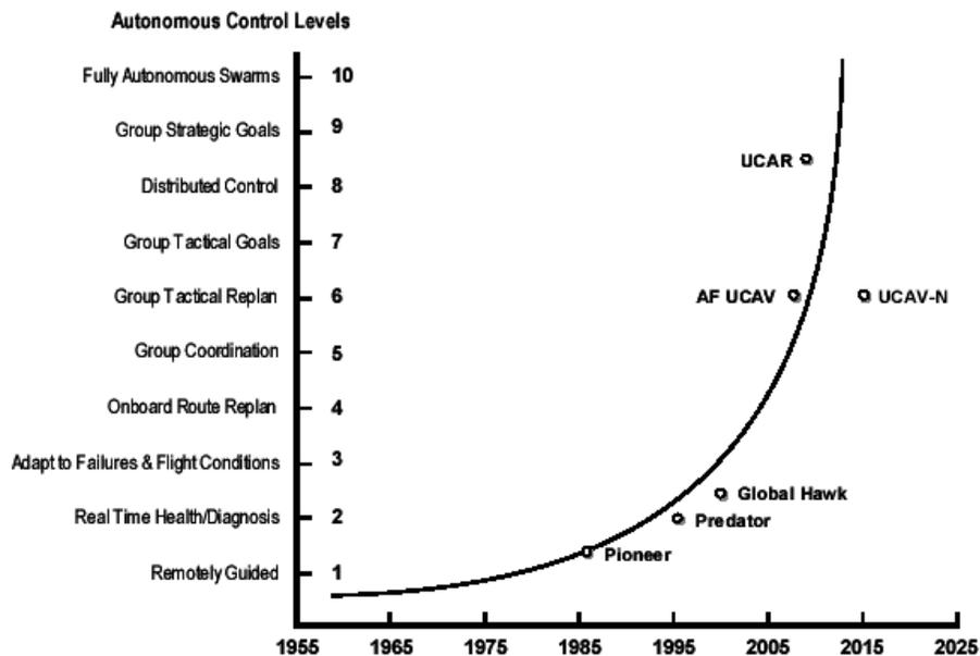
The above chart is from the UAV Roadmap prepared by the UAV Planning Task Force. The curve shows availability of total autonomy by 2015 although no fully autonomous systems are shown as being deployed.
